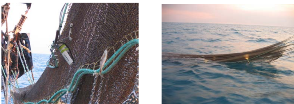
Fig 4. The battery pod attached to the sled and a light mounted on the headline ( left ). The illuminated trawl net at the surface ( right ).
