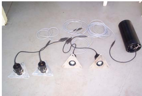
Figure 1: A representative light system as used in the field trials. The battery pod (right) is cabled to each of the lights. Each light is attached to a mounting bracket, allowing the lights to be uniformly attached and orientated.
