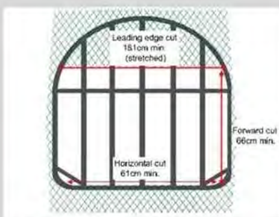
Figure 7: Required dimensions for rectangular opening
