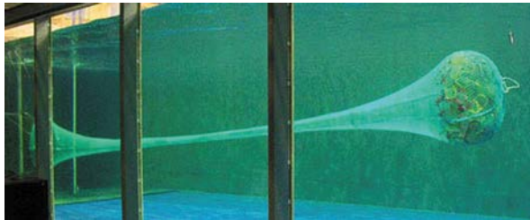
Above: Traditional codend. Notice the mesh is pulled in, reducing the opening.
