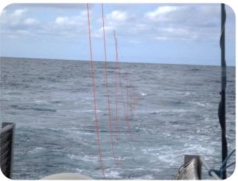
Examples of effectively designed and deployed tori lines (Photos: AFMA observers)
