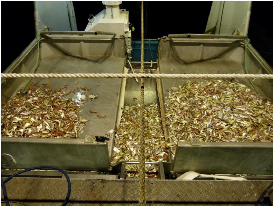
Figure 4: Catch from the net with the Kon's Covered Fisheyes BRD (left) compared to a control net with a Square Mesh Panel BRD (right side), excluding the catch on the conveyer in the center. When compared, these two codends had the same quantity of prawns but significantly less bycatch in the net with the Kon's Covered Fisheyes BRD.
