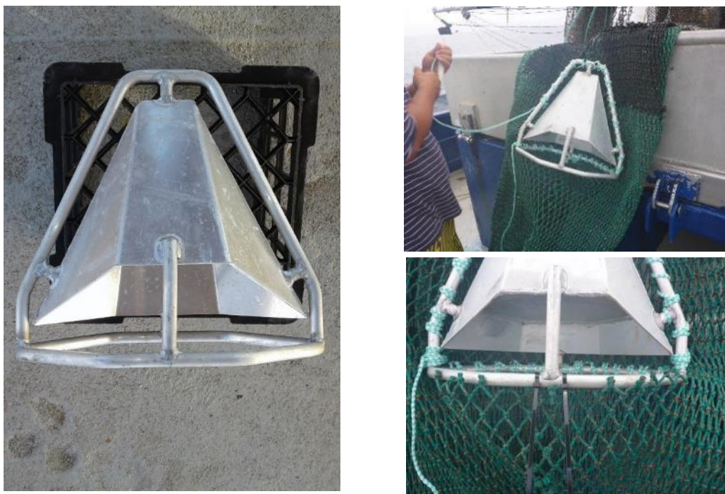
Figure 2: Tom's Fisheye without cone back plate (left) and modified with cone back plate (right) (source: A. Raptis & Sons P/L).
