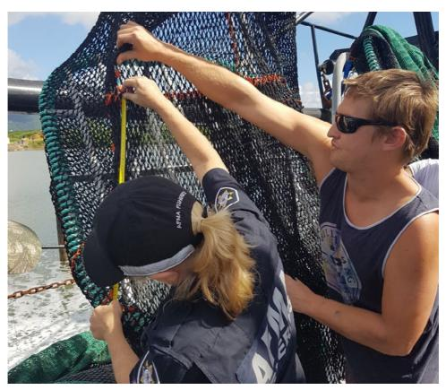
Figure 10: Dylan Prendergast (Austral Fisheries) helps Janet Norenbergs (AFMA) to measure a turtle exclusion device.
