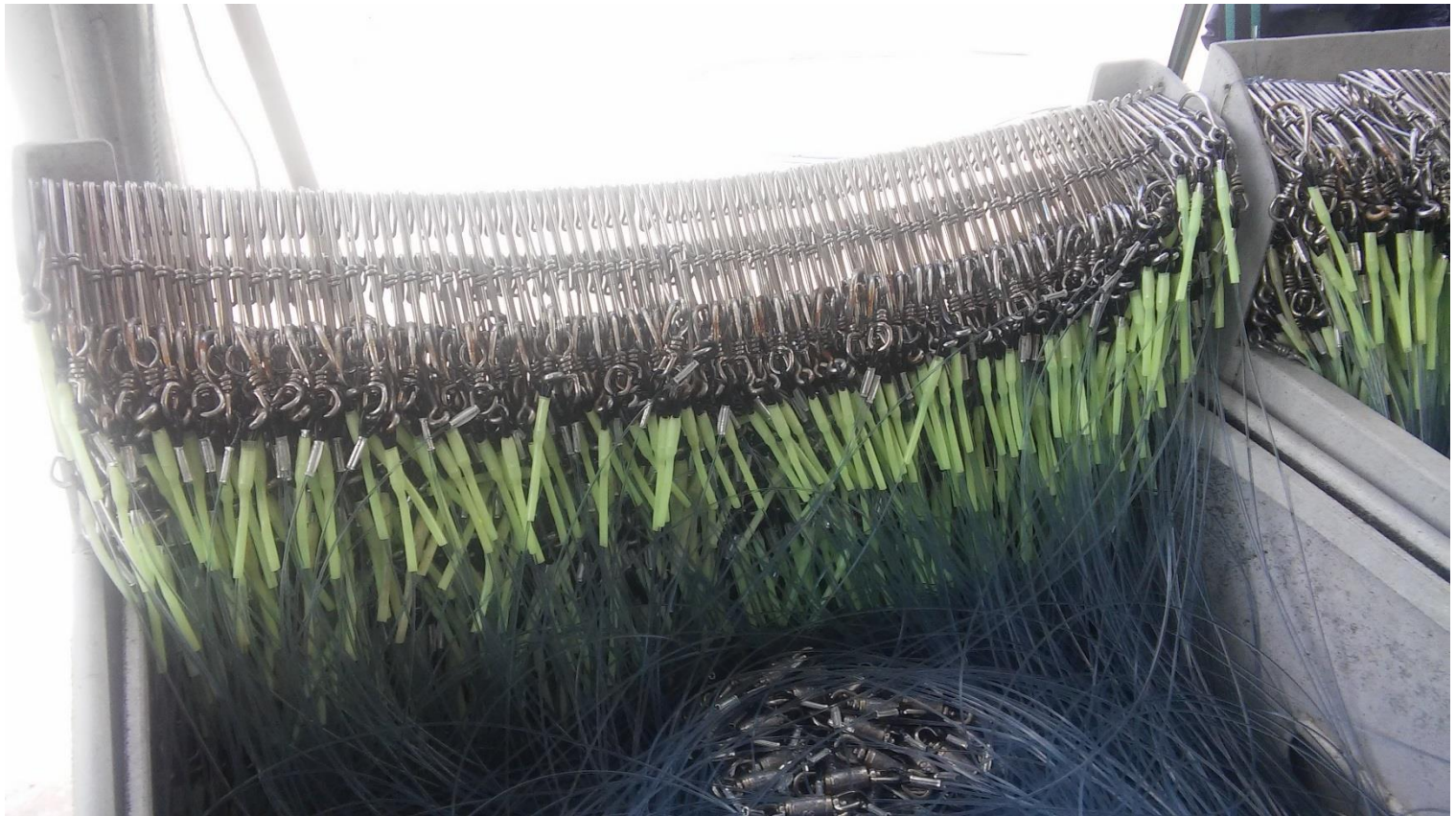
Image. Manual longline hook setup
