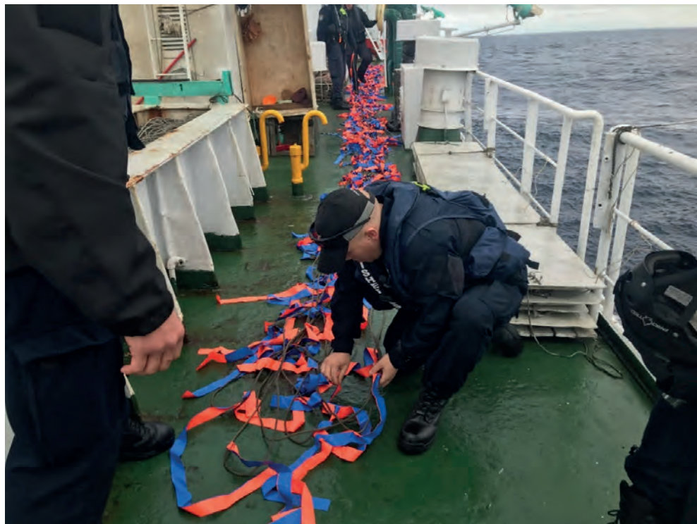
Multilateral Operation Operation Nasse – an AFMA officer inspects a tori line (used to scare seabirds away from baited hooks) during fishing on board a foreign flagged longliner Photo courtesy AFMA
