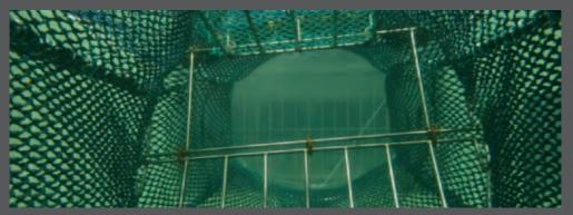
AFMA staff have worked in partnership with industry during 2010-11 to develop the "TuddySED", an acoustically triggered seal excluder device.
