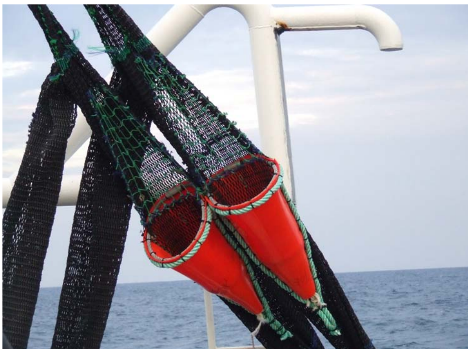
Figure 4. Witches hat BRD enhancers in port side nets.
