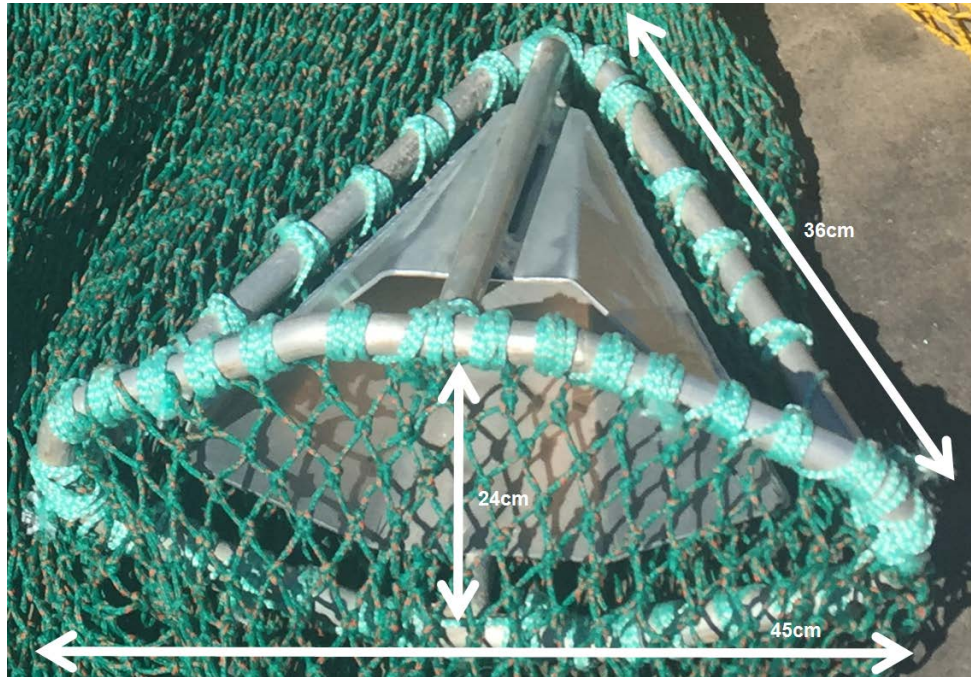
Figure 1: A single Kon's Covered Fisheye stitched into the net including device specifications. The device was 45cm in total width, but the inside width of the mouth was 37cm.
