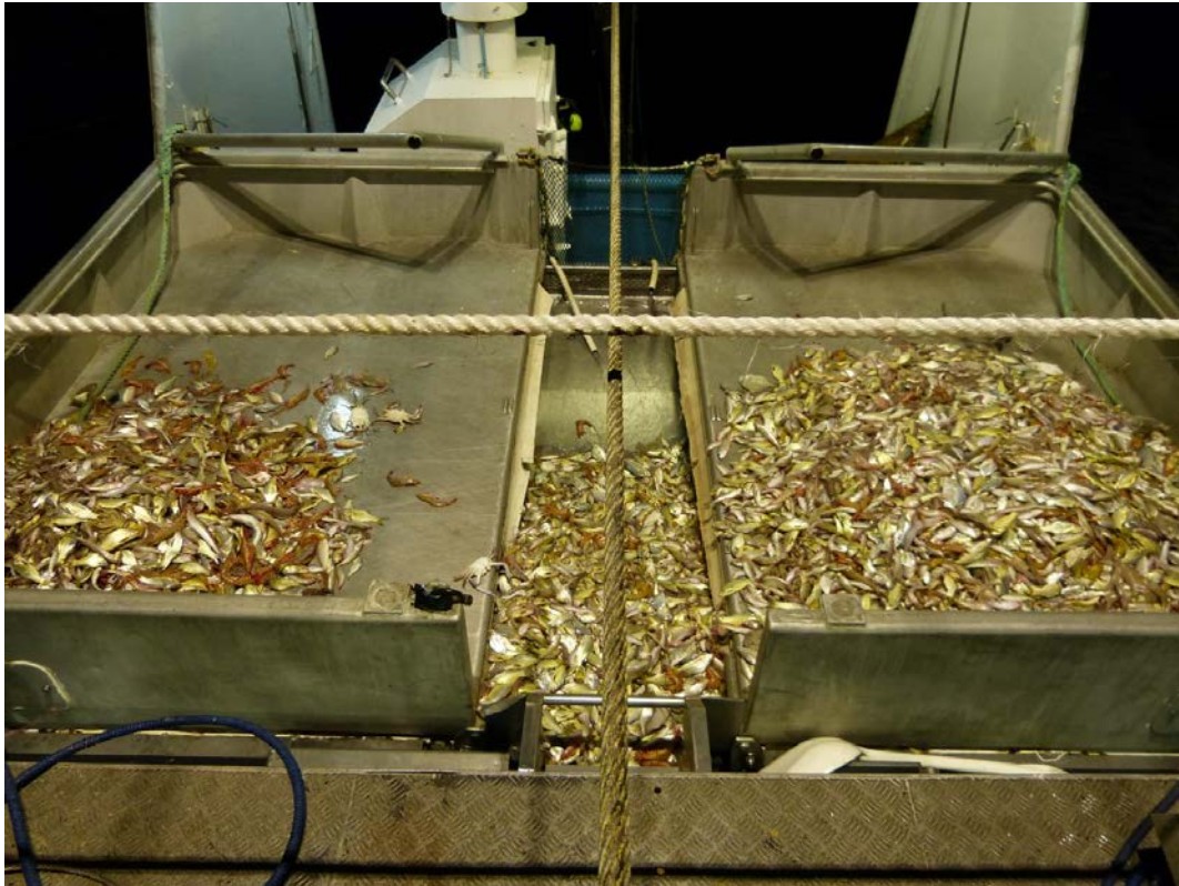
Figure 3: Catch from the net with the Kon's Covered Fisheyes BRD (left) compared to a control net with a Square Mesh Panel BRD (right side), excluding the catch on the conveyer in the center. When compared, these two codends had the same quantity of prawns but significantly less bycatch in the net with the Kon's Covered Fisheyes BRD.
