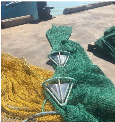
Kon's Covered Fisheye's stitched into net Photo courtesy: AFMA
