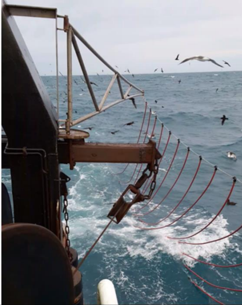
FV Western Alliance with bafflers deployed whilst fishing
