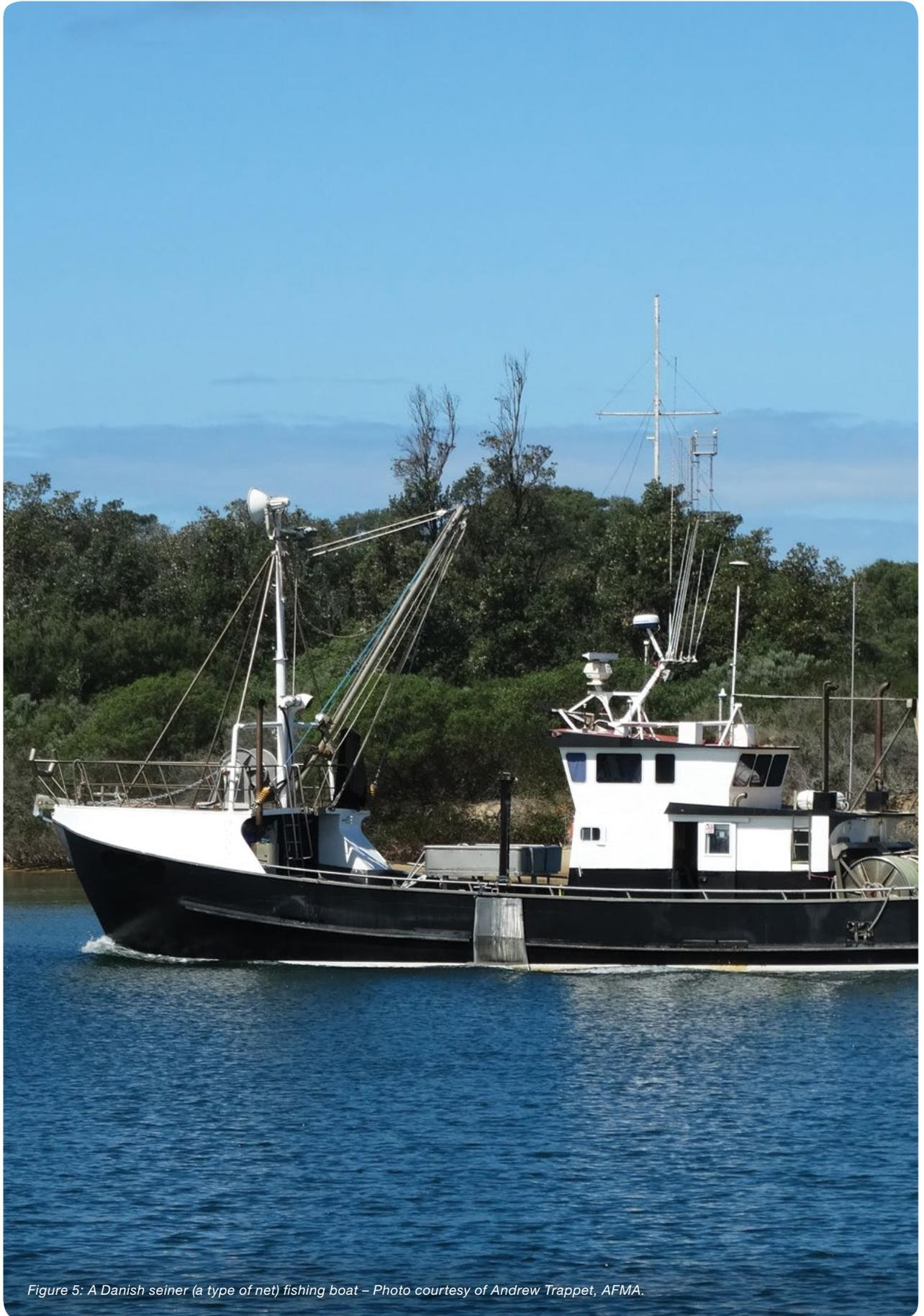
*Figure 5: A Danish seiner (a type of net) fishing boat – Photo courtesy of Andrew Trappet, AFMA.*
