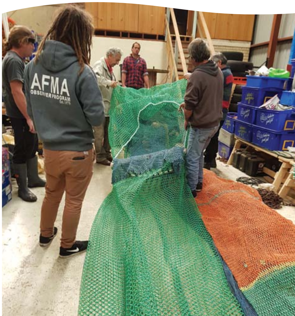
AFMA and industry discussing installation of Gulper Shark Exclusion Device on South East Trawl boats
