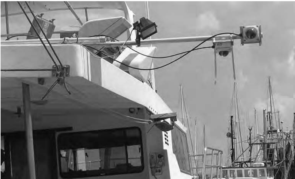
Newly fitted e-monitoring cameras on a vessel in the Eastern Tuna and Billfish Fishery. A trial of e-monitoring is currently underway in this fishery. Photo – Matt Piasente.
