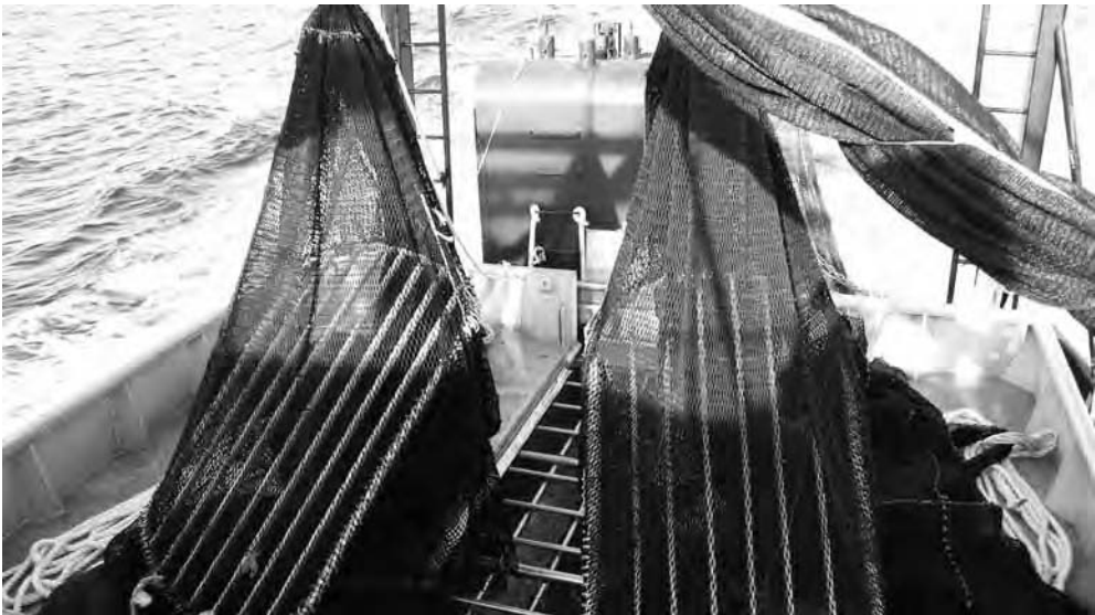
Turtle Excluder Devices, such as these being used in the Northern Prawn Fishery, allow turtles and other non-target species, including threatened, endangered and protected species, to escape trawl nets. Minimising the impacts of fisheries on the marine ecosystem is one of AFMA's key legislated objectives and an important part of ensuring AFMA meets its obligations under the Environment Protection and Biodiversity Conservation Act 1999 . Photo – AFMA
