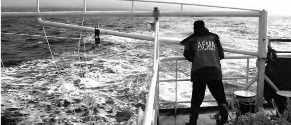
An AFMA Observer monitoring setting of tori lines in the Macquarie Island Toothfish Fishery. Tori lines are used to discourage seabirds from attacking baited longlines during the setting of gear. This is an important initiative to prevent incidental mortality of endangered species in Australia's southern oceans fisheries and no seabird interactions have been reported in the fishery for four years. Photo – Sam Hyson
