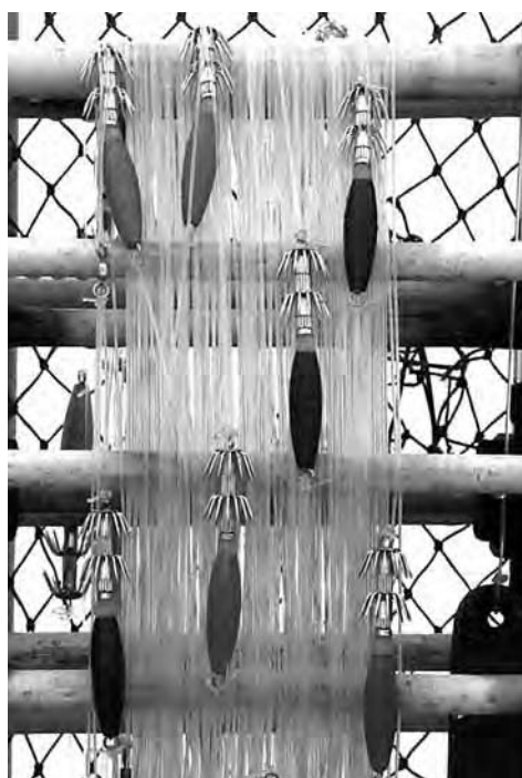
Squid jigging equipment on a Southern Squid Jig Fishery vessel in Portland, Vic. Photo – Matt Daniel
