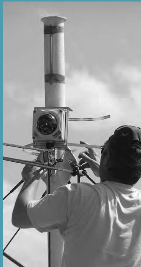
Electronic monitoring equipment, such as the camera shown being mounted onto a fishing vessel, has the potential to provide a cost-effective at-sea monitoring option. Photo – Matt Piasente
