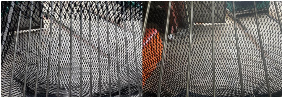
Figure 7: The smaller bar spaced TED has a 70 mm width (SBS-70-TED) between bars (left photo) while the standard TED has a 110 mm width (right photo).
