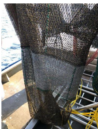
Figure 24: The experimental 30-mesh grey magnet material throat section Flinders Pearl.
