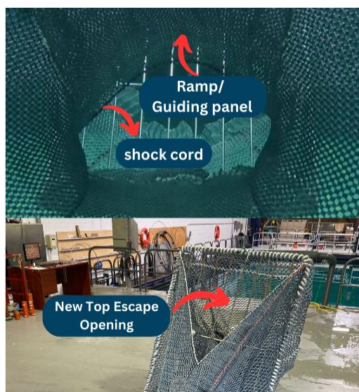
Figure 1: The ramp guiding funnel and the elastic shock cord used to direct the catch down toward the STED.
