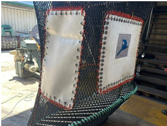
Figure 17: Composite fabric material installed in patches near the TED.
