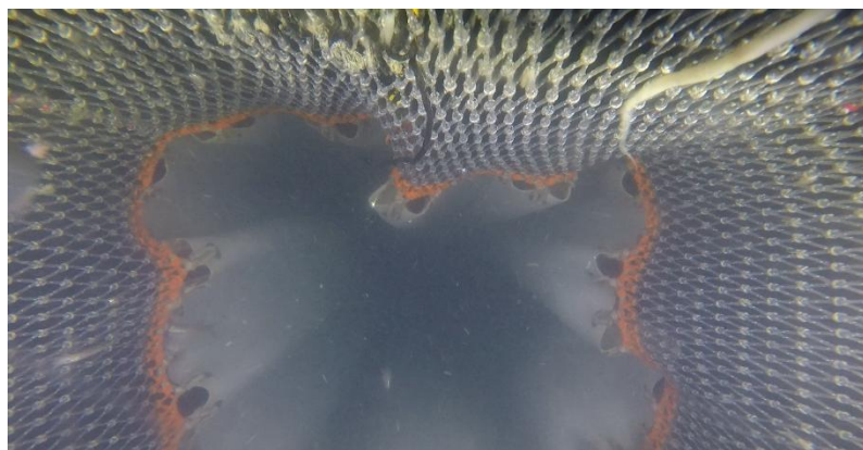
Figure 19: Composite canvas material throat sock (FloMo) trialled onboard the Kodiak T tiger prawn season 2024.
