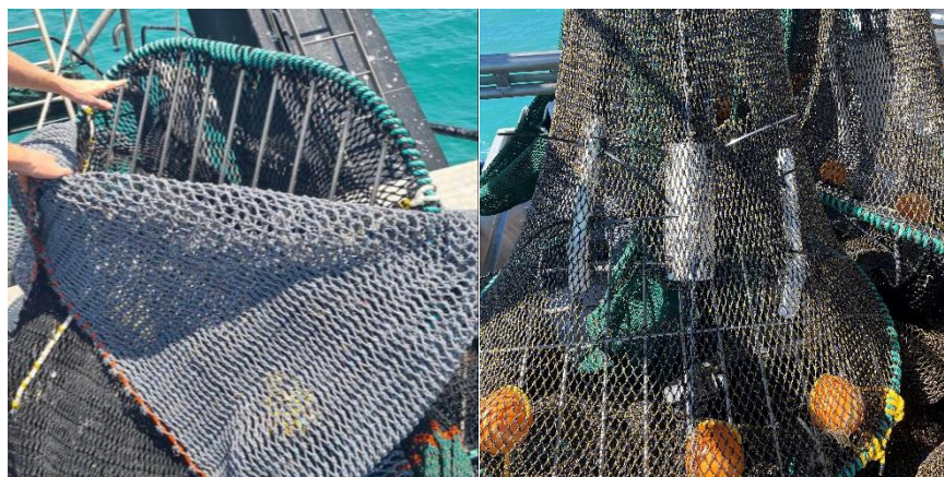
Figure 11: Grey Magnet Mesh TED flaps with underwater camera and two lights installed 600 mm behind the TED.
