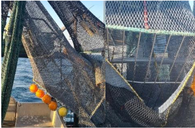
Figure 5: STED installed port side to compare prawn catch, sawfish interactions and bycatch differences against standard TED's.
