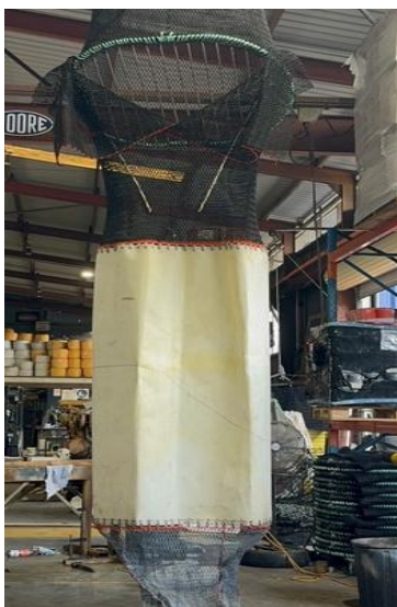
Figure 18: Composite fabric material (FloMo) inserted in the throat section of the net.
