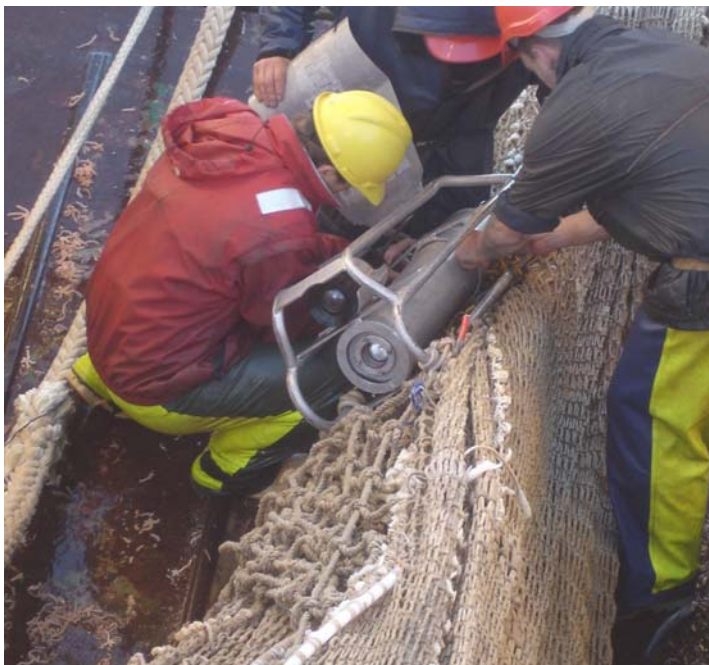
Fig. 1: The crew of the Ellidi lashing the camera system to the trawl net, adjacent to the escape opening of the exclusion device.
