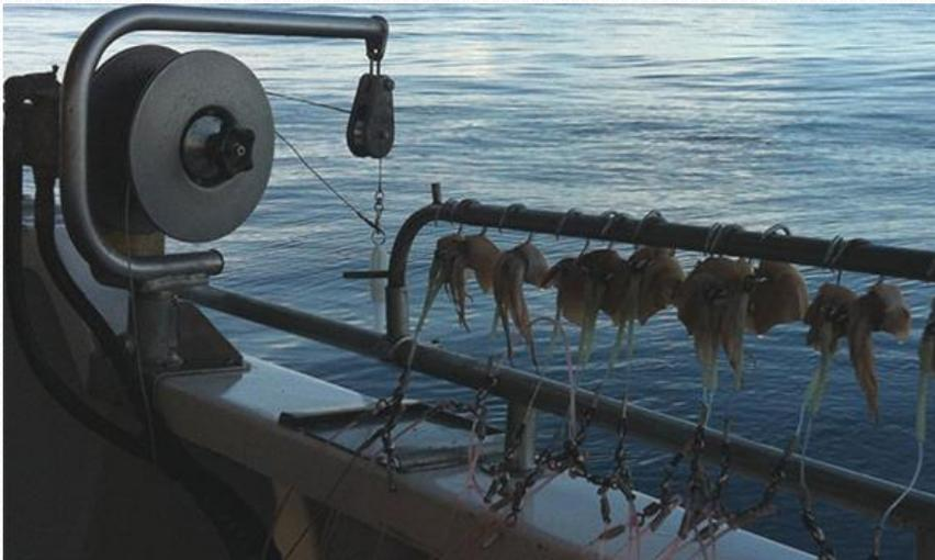
Hydraulic line hauler for deepwater fishing for wreckfish
